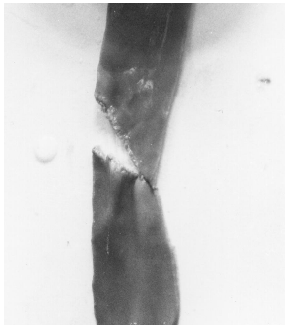
Figure 4 Illustration of how cutting stress is produced (breaking point).
